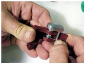
4) Position tool and lock lever on the top of the post. Push lever onto post until it stops. Pull the tool out of the lock lever, holding the lever and spring on the coupling. Push lock lever the remainder of the way onto the post.
