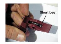
2) Align the flat on the peg with the flat inside of the locking lever hole. Slide locking lever and spring onto tool. There are two small pins and one large pin on the tool. When the tool is properly placed on the locking lever the two small pins will be on opposite sides of the lever part of the locking lever
