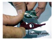
3) Place long leg of spring under pin on the tool and push tool completely onto the locking lever. This will preload the spring. The locking lever is now ready for installation on the coupling.
