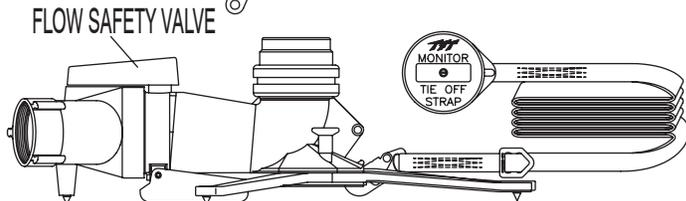
The **STOW-A-WAY 800 PORTABLE BASE WITHOUT SAFE-TAK VALVE** is supplied with either two clappered swivel inlets or with a single full-time swivel inlet. Includes a safety tie-down strap with attached storage cap. STOW-A-WAY 800 portable base is not equipped with SAFE-TAK™ "Flow Safety Valve." Maximum recommended flow with Stow-A-Way Base in portable mode is 800 gpm (3500 l/min). Order XF500-KIT Option \$500.00 to add a flow safety valve. Weight of safety valve is 3.1 lb (1.4kg).
