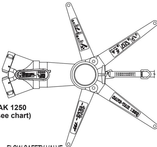
**SAFE-TAK 1250 PORTABLE BASE WITH SAFE-TAK VALVE** is supplied with either two clappered swivel inlets or with a single full-time swivel inlet. The stainless steel, carbide-tipped base support legs can be folded to easily fit inside a small apparatus compartment, or for carrying pre connected to a hose line. Includes a safety tie-down strap with attached storage cap.
