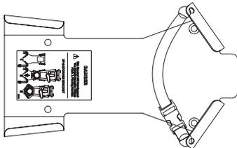
**XF-B** - CROSSFIRE STORAGE BRACKET A 13 ga., 304 stainless steel bracket with strap holds the Stow-A-Way 800 or the Safe-Tak 1250 portable base securely while being transported. This 14.75" x 7.75" x 2" (37.5 x 19.7 x 5.1cm) bracket can be mounted vertically or horizontally in any position, including the top or underside of a shelf, on a side wall, or on a compartment door. Includes quick release storage strap.
