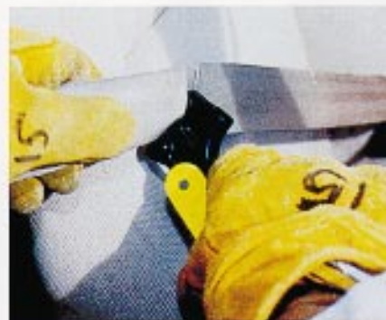
Seatbelts cut easily with the tool's sharp edge.
