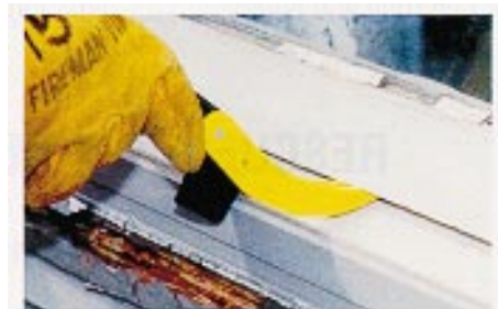
With the Res-Q-Rench, firefighters no longer need a crowbar to pry open a window.
