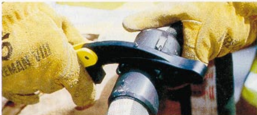
The tool makes it easier to connect a hose coupling.
