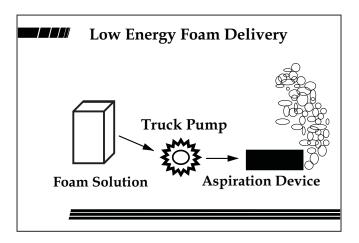
Low Energy Foam Delivery Systems, or nozzle aspirated foam, take the energy from the horsepower of the truck engine, transferred through the fire pump, throughout the hose line to the end of the line at the nozzle.
