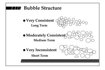
The Structure of bubbles in the finished foam blanket can best be tactically characterized in three categories:
