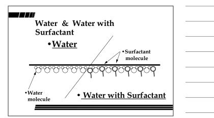
Hydrocarbon surfactant molecules tend to be water shedding and oil loving.
