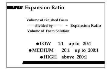
Since it takes energy to produce a finished foam, it follows that, the more energy used to aspirate foam solution, the higher the volume of finished foam.
