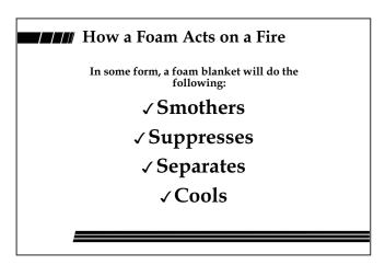
**Smothering** - The use of a foam blanket will provide an excellent covering that can be used to surround a fuel thereby breaking a side of the tetrahedron. This smothering ability will act to isolate the fuel from other sides of the tetrahedron.
