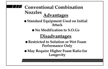
Though 95% of initial attacks on structural fires use the first two lines off the engine, these limitations have not been greatly discussed. On initial interior attack, extensive foam creation is not necessary. The "wet" solution type of foam is ideal for the soaking and coating need of this type attack. Overhaul operations actually begin upon initial attack. The soaking ability immediately reduces the opportunity for rekindle.
