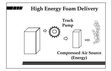
High Energy Foam Delivery Systems, or CAFS (compressed air foam systems), do not use the energy transferred to the hoseline from the fire pump. Instead, a third component, an air compressor, is mounted on board the apparatus and adds compressed air (energy) in the form of pressure (psi) and flow (cfm). This energy is transferred into the hose line, which holds it in the form of stored energy awaiting release at the tip.
