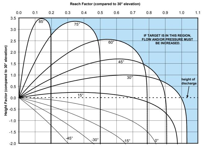
Stream reach and height at non-optimal elevations can be estimated as a factor of the performance at the optimal 30° elevation. Refer to LIM-030 and LIM-035 for effective stream trajectories of Task Force Tips Masterstream nozzles at 30° elevation. This graph cannot be used to estimate maximum reach for elevation angles below 30°.
