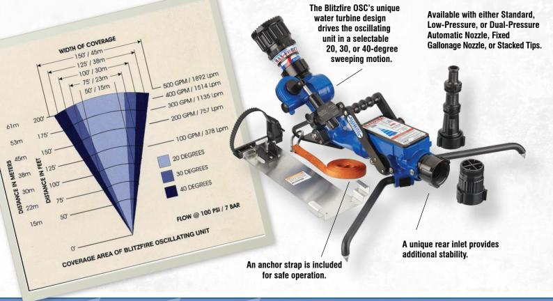
With a flow range up to 500 gpm (2000 lpm), the Blitzfire HE OSC portable monitor features low loss pivoting inlets and outlets, as well as a manually adjustable elevation from 10 degrees up to 86 degrees. The integrated water driven oscillation mechanism sweeps in a selectable 20, 30, or 40-degree pattern for maximum exposure coverage. The standard safety shut-off valve will shut off if the monitor becomes unstable. Slow valve closure design diminishes potential
