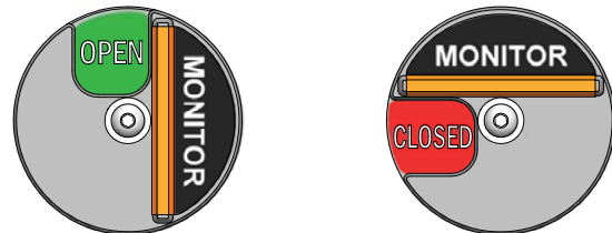
Figure 5.1.2: Monitor valve position indicator (orange flag)
