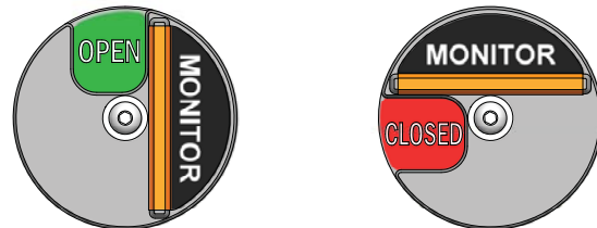
Figure 5.1.2: Monitor valve position indicator (orange flag)
