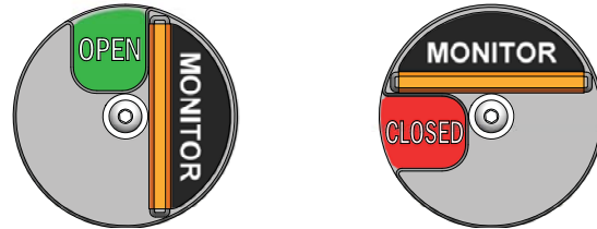
Figure 5.1.2: Monitor valve position indicator (orange flag)
