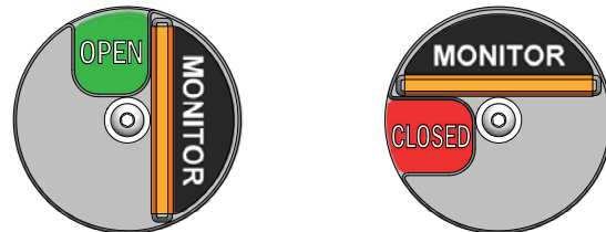
Figure 5.1.2: Monitor valve position indicator (orange flag)
