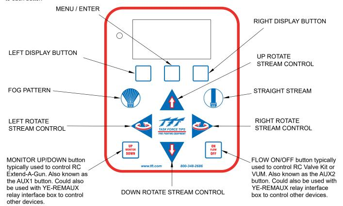
Figure 3.0 Operator Station with Display Control Pad
