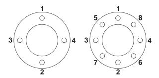
Figure 4.1 Flange Bolt Tightening Sequence
