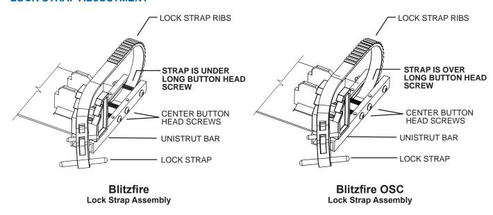
To adjust the tension of the lock strap (13), remove the two center 1/4-20 x 2" button head screws (16) that retain the lock down assembly. Change the position of the lock strap ribs in the unistrut bar (11). Reinstall the cap button head screws (16) and cap nuts (15) and tighten. Check the tension of the strap when the Blitzfire is mounted. Readjust tension if necessary.
