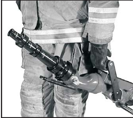
Figure 4.1 Carrying the Blitzfire on an Uncharged Hose
