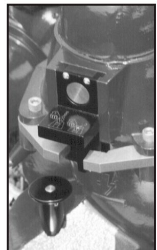
Figure 4.4.3 Slide bar locked, safety plunger is engaged
