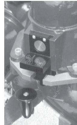
Figure 5.4.3 Slide bar locked, safety plunger is engaged
