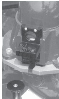
Figure 5.4.2 Slide bar up, safety plunger is not engaged
