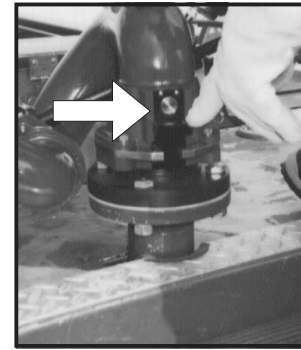
Figure 3.2.3 Slide bar locked, safety plunger is engaged.
