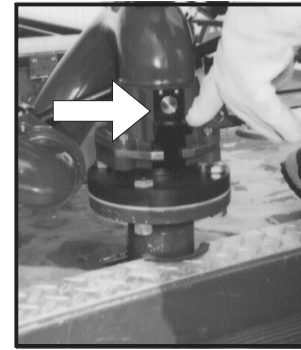
Figure 3.2.3 Slide bar locked, safety plunger is engaged.
