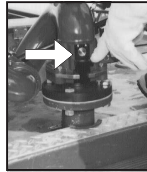
Figure 3.2.3 Slide bar locked, safety plunger is engaged.
