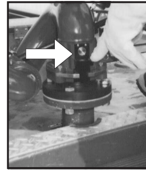
Figure 3.2.3 Slide bar locked, safety plunger is engaged.
