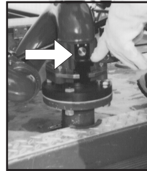
Figure 3.2.3 Slide bar locked, safety plunger is engaged.
