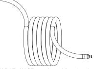
DISCHARGE HOSE — for adding length between the PRO/pak and the nozzle for maneuverability. Maximum distance is 25 feet (7.6m). Quick connect 3/4" (19mm) hose has a 300 psi (21 bar) pressure rating.
