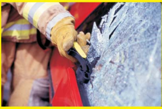
With its integrated carbide tip window punch, the Res-Q-Rench can quickly pop out windows during vehicle extrication.
