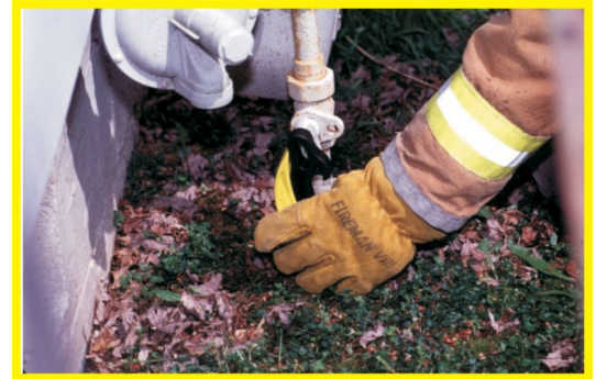
The Res-Q-Rench has an integrated shut-off which fits many residential gas valve
