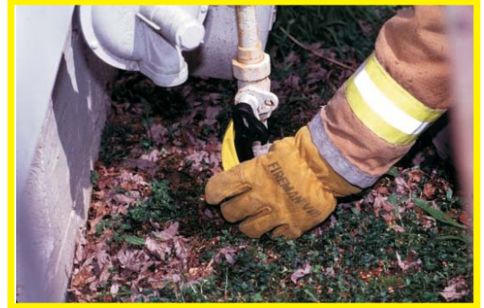
The Res-Q-Rench has an integrated shut-off which fits many residential gas valve
