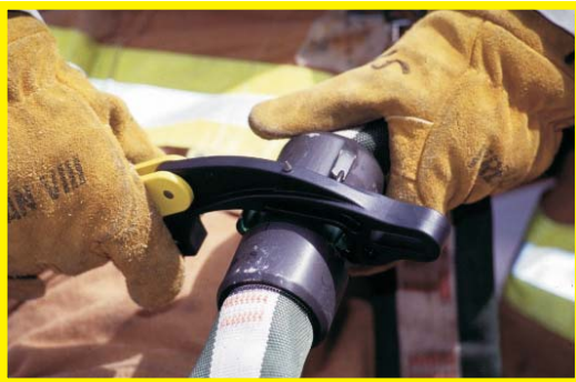
The Res-Q-Rench is designed to work with rocker lug handline and supply line couplings and is the only folding spanner that will work with 4" and 5" storz locking couplings.
