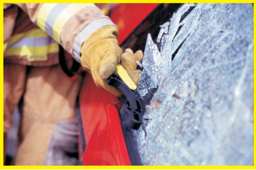
With its integrated carbide tip window punch, the Res-Q-Rench can quickly pop out windows during vehicle extrication.
