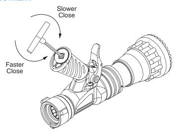
Do not unscrew the adjuster past the end of the hand grip (to unscrew it too far could result in the loss of dampening fluid.)
