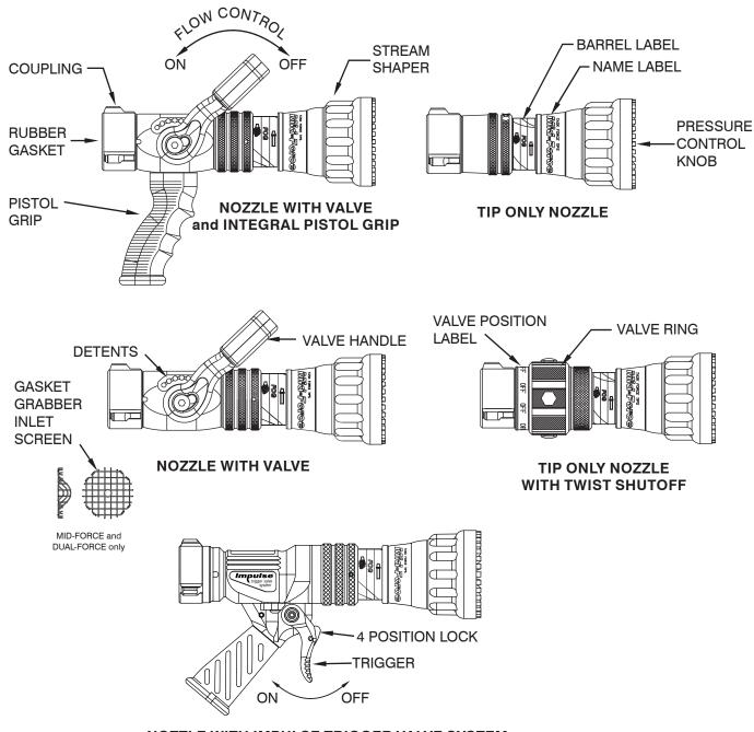
**NOZZLE WITH IMPULSE TRIGGER VALVE SYSTEM**
