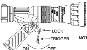
NOTE: THE TRIGGER RETURNS TO OFF IF NOT HELD OR LOCKED
