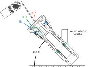
While holding nozzle at the angle, wait 30 seconds for the lubricant to penetrate into the clearances. Cycle the valve handle and rotate the shaper from straight stream to full flush several times, and then proceed to the next section.
