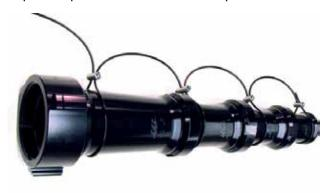
**6)** Snug each loop around tip such that cable rotates around tip freely, but does not slip off tip. Tighten all screws.
