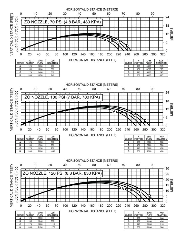
Fig. 3.2 Stream Trajectory Data
