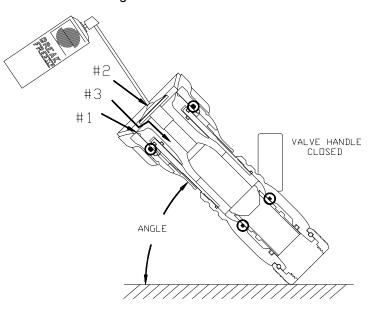
While holding nozzle at the angle, wait 30 seconds for the lubricant to penetrate into the clearances. Cycle the valve handle and rotate the shaper from straight stream to full flush several times, and then proceed to the next section.
