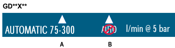
Figure 4.4D 1.0" / 25 mm G-Force 75 psi / 5 bar Automatic with Flow Limiting
