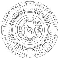
This model, and all versions of the Dual-Force, offers the unique ability to change operating pressures at the nozzle. This allows greater flows at a lower operating pressure when needed.
