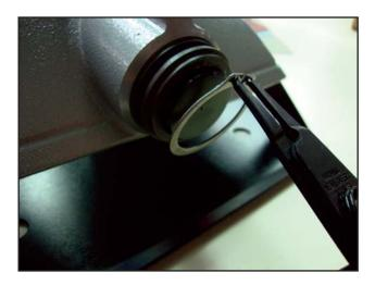
1.2 Apply a layer of grease (VSA-104) to the o-ring grooves in the Adapter, install O-rings and apply a layer of grease over it.
