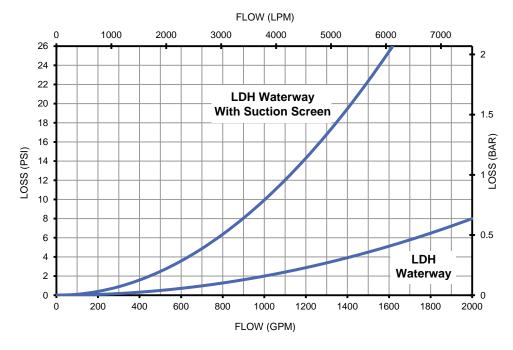
Figure 5.4 Pressure Loss Chart
