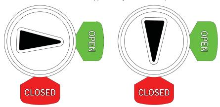
Figure 5.1 Valve Position Indicator
