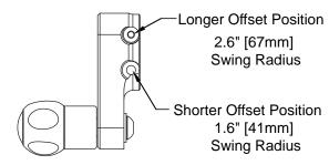
Figure 4.2 Crank Handle Offset
