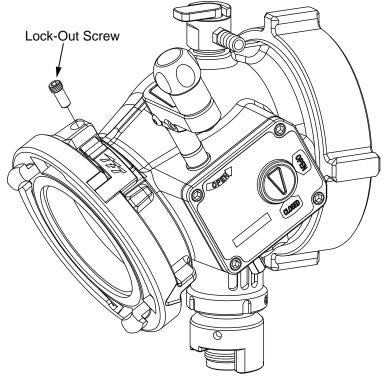
Figure 4.3. Coupling Lock-Out
