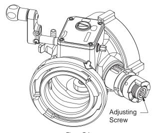
Figure 7.1 Pressure Relief Valve
