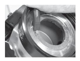
2) Unscrew and remove seal retainer.
