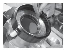
6) Grease the backside of the seal.
