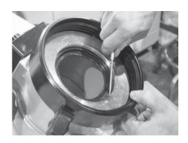
5) Use a pointed pin to make sure the corner of the rubber seal does not hang up on the edge of the threads. Run the pin around the outside edge of the seal. Make sure the pin does not create a large gouge in the seal.
