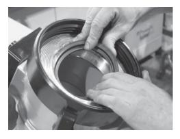
4) Install the new Valve Seat into Back Ring. The lip on the seal goes in first.
