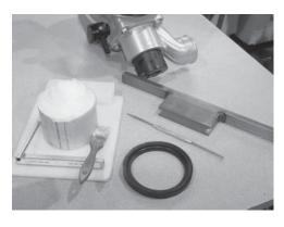
Needed: new valve seat, small amount of white grease, a pointed pin, wrench, Tool #THA406 and seal retainer remover tool (available from tft if needed).
