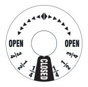
**6.0 AIR VENT AND WATER DRAIN**This valve is equipped with an Air Vent/Drain which will allow the air to escape from the valve when the hose is charged. The Air Vent/Drain is opened by turning the knob counter clockwise and closed by turning it clockwise.
