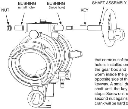
The handwheel is shipped from the factory on the right hand side of the valve. The hand wheel. can be switched to the left hand side for convenience or if it interferes with other equipment on the pump panel.
