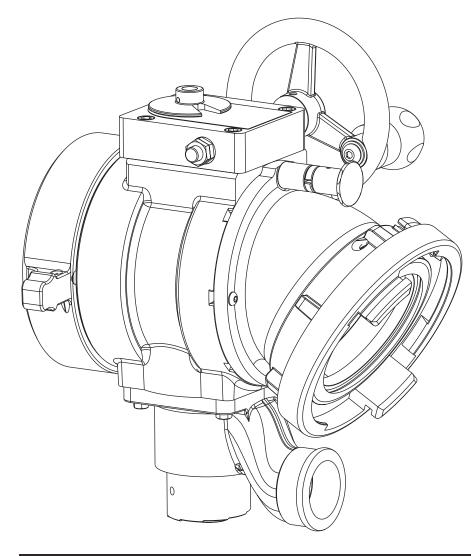
**OPERATING RANGE:** Pressure Max 250 PSI Pressure Min Full Vac.
