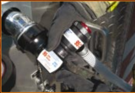
New eductors available with either 2 1/2" or 1 1/2" inlet
