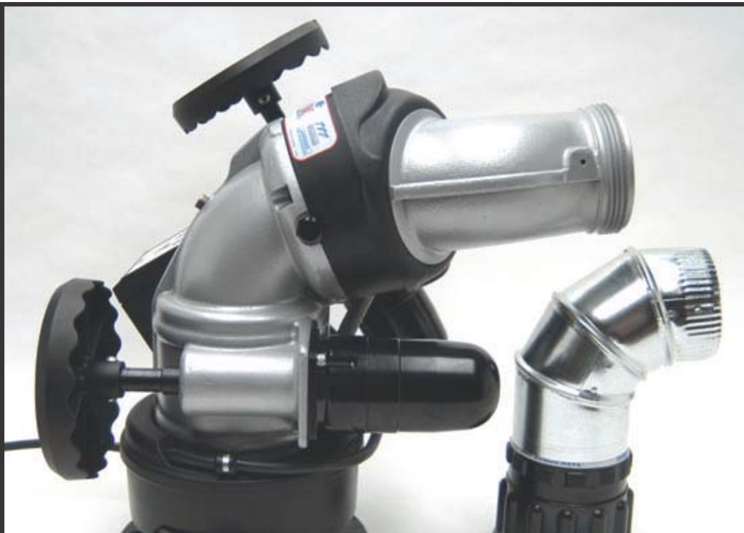
A simple stovepipe elbow inspired the concept for TFT’s new monitors. A double swivel joint helps reduce the number of sharp 90-degree bends that cause friction loss in other monitors. (Fire Apparatus Photo by TFT)
