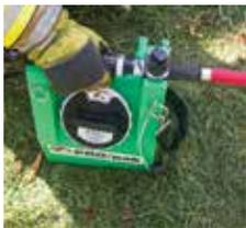
Flow is controlled by a twist grip valve. Cleaning agents are added through the large, easy-open fill port that includes a debris screen.
