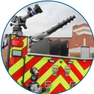
RC Monitor and Ball Intake Valves
