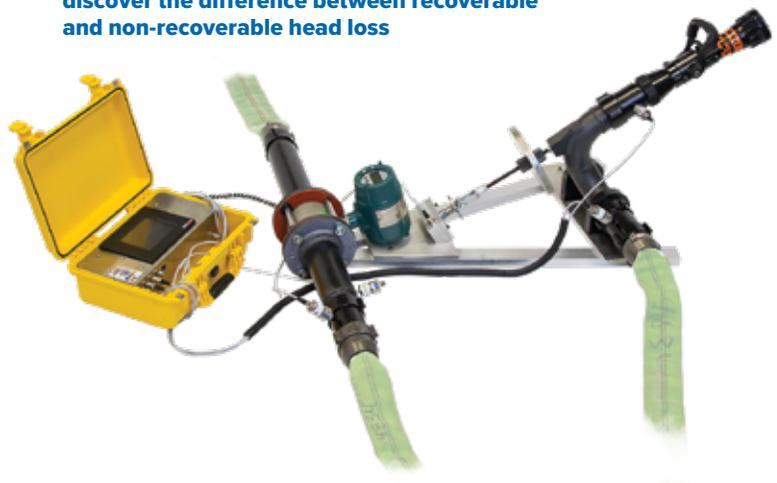
**MEASURE AND COMPARE:** Nozzle Pressure, Reaction Force, Friction Loss, Stream Straighteners and Head Loss
