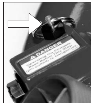
Figure 4.5.3 Elevation stop pin in
