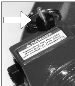
Figure 4.5.2 Elevation stop pin out
