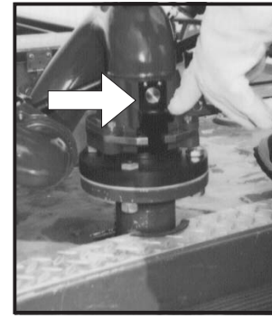
Figure 3.2.3 Slide bar locked, safety plunger is engaged.
