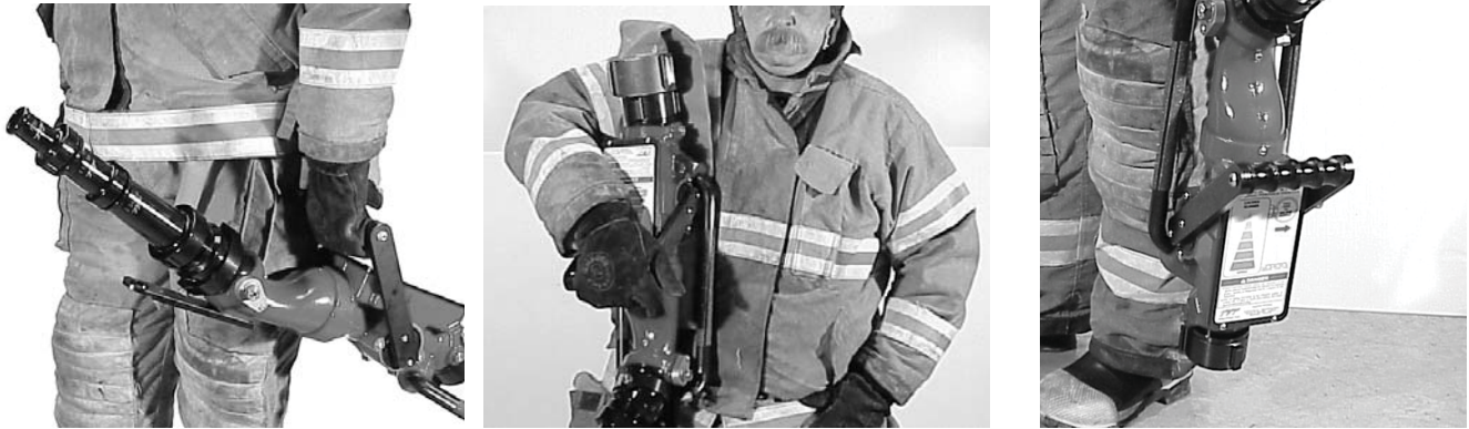
Figure 4.1 Carrying the Blitzfire on an Uncharged Hose
