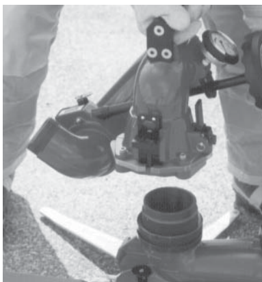
Figure 5.4.1 Hold monitor by the top carrying handle, position monitor over base and slide straight down
