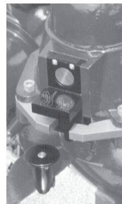
Figure 5.4.3 Slide bar locked, safety plunger is engaged
