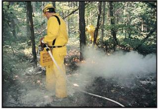
The PRO/pak makes foam and limited water supply go further. Low expansion nozzle makes wet and sloppy foam to penetrate burning Class A materials. Medium expansion nozzle provides longer-lasting, thick, shaving-cream-like foam for pretreatment ahead of a fire front.
