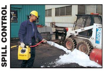
For a liquid hazardous material spill, the Pro/pak can be used with either 1% or 3% CLASS B Foams. The PRO/pak is simple to operate and dependable under a variety of conditions. For vapor mitigation, the Medium Expansion foam attachment produces highly expanded foam to suppress vapors and reduce the possibility of ignition.
