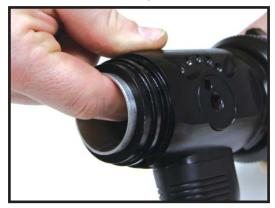
3701 Innovation Way, Valparaiso, IN 46383-9327 USA 800-348-2686 • 219- 462-6161 • Fax 219-464-7155 **Step 7)** Inspect the tapered leading edge of the slider. This is the edge that seals against the plug. If this edge is damaged replace the slider. (Part # G605)
