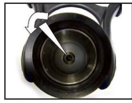
**Step 19)** Included with the kit is a new o-ring (VO-222) to seal the coupling to valve body connection. Lightly grease this o-ring. Install this o-ring on the valve body as shown. Also, lightly grease the ball ring groove on the valve body.
