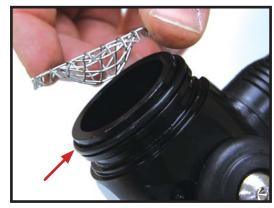
**Step 20)** Install the debris screen over the valve body so the concave portion faces down over the valve body. Next, lightly and evenly press the coupling down onto the valve body. Pay close attention that the o-ring does not get pushed out of place or pinched.
