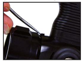
**Step 2)** Holding the nozzle over a container with the port plug hole facing down rotate the coupling until all the ball bearings fall out. 33 balls retain the coupling. Once all the ball bearings have been removed pull off the coupling, debris screen, and o-ring.
