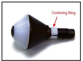
**Step 11)** Thread the new valve plug into the valve body until snug. DO NOT tighten.
