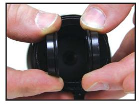
**Step 14)** Lightly grease the outside circumference of the slider with the grease provided in the kit. Install the slider with the chamfered edge facing the valve plug. Use caution when installing the slider that it does not pull the valve discs out of place. Push the slider in until it contacts the valve plug then pull back about 3/8".
