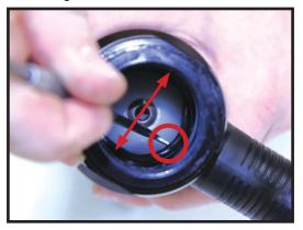
**Step 9)** Using the 3/16" Allen wrench, un-thread the valve plug from the valve. The green aluminum center will accept an Allen wrench.
