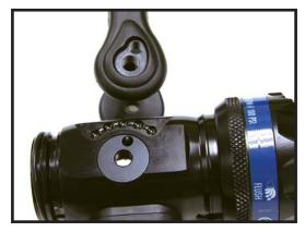
**Step 17)** Install a cam pin in each cam pin hole. Insure it seats in the groove in the slider. The cam pin face should be flush with the surrounding handle when properly installed. Apply red Loctite® to the threads of the button head screws that retain the handle. Install one on each side of the handle until hand tight.
