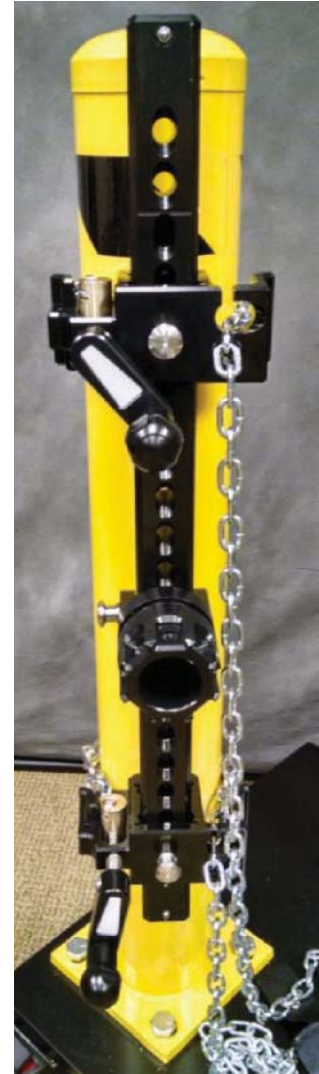
La Figure 2.30 Installation du support de tige transversale
