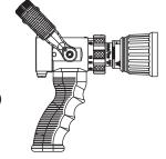
**DQS60P** QUADRAFOG W/GRIP 1" NH (25mm) - Selectable gallonage nozzle with five flow settings of 5, 10, 24, 40 and 60 gpm @ 100 psi (20-40-90-150-230 l/min @ 7 bar). All lightweight materials, hardcoat anodized aluminum. Flush without shutting down. Quick-change rear valve seat and stainless steel shut-off ball. Pistol grip is mounted below the valve. Rocker lug 1" NH swivel is standard.
